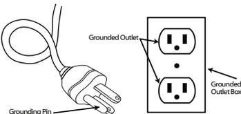
This product is for use on a nominal 120-volt circuit and has a grounding plug that looks like the plug illustrated in sketch (A). Make sure that the product is connected to an outlet having the same configuration as the plug. No adapter should be used with this product.
